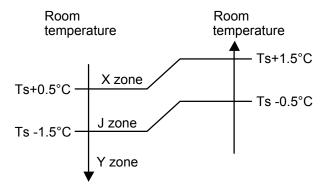
(Fig.4: Indoor Fan Control)
