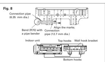
After hooking the indoor unit to the top hook, hook the fittings of the indoor unit to the two bottom hooks while lowering the unit and pushing it against the wall.
